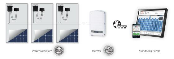
\* SolarEdge power optimizers can operate with any inverter.
