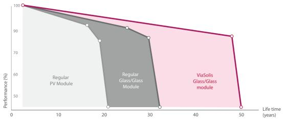
Thanks to ViaSolis unique lamination technology based on long-term experience of Automotive and Glass processing industries, the ViaSolis module ensures excellent power output and stable yields over the 50 years exposed at extreme conditions even.\*
