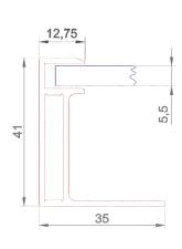
Note: Dimensions are given in millimeters
